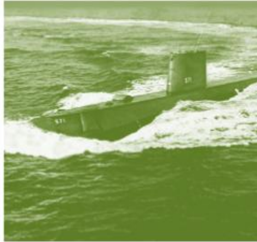
Nautilus 10 MWe First ever PWR Electric Boat full scale prototype 1949 + 4+2 years
